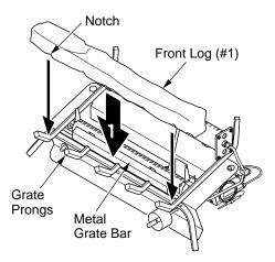
Figure 21 - Installing Front Log (#1) [18" Variable Manually-Controlled Set Shown]
